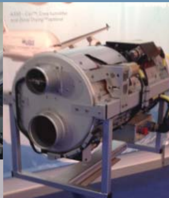
Dehumidifier for a 737 takes out the water buildup from condensation in the ceiling blankets, saving fuel by reducing the weight of the water getting absorbed into the blankets.
