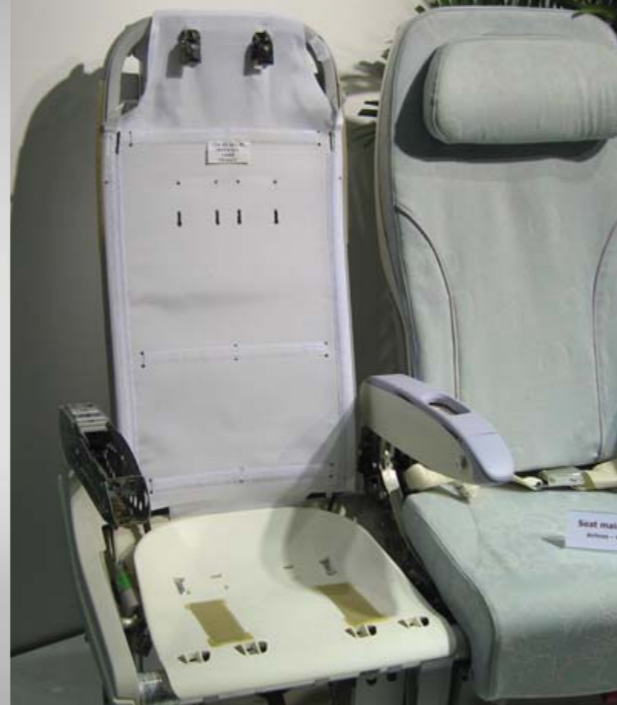
Composite materials to lighten weight of seat frames
